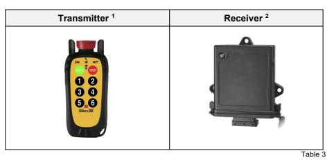
The emergency stop function provide a stop category 0 according to EN 60204-1:2018 § 9.2.2. The reliability of the emergency stop function was evaluated to fullfil the safety requirements for the performance level "pl d" according to EN 13849-1:2015 § 4.5.1.
